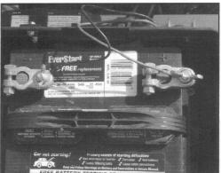
5. Connect battery wires: RED to + and BLACK to - (Battery not included)
