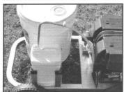
**8.** When finished marking your field, take the pick-up tube out of the 5 gallon bucket and put it in the 1 gallon container of water. Continue to mark an existing line until the system is **COMPLETELY FLUSHED OUT.**
