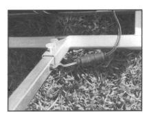
6. Slide handle into square tube on the back of the machine and tighten the thumb screws. Attach electrical plug and turn on switch near top of handle to start.
